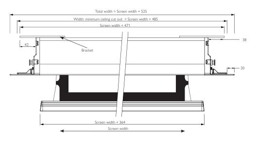
Considerations regarding cut out width Minimum cut out width: screen width + 485 Maximum cut out width: screen width + 523 Recommended cut out width: screen width + 505
