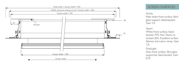
Considerations regarding cut out width Minimum cut out width: screen width + 305 Maximum cut out width: screen width + 343 Recommended cut out width: screen width + 325
