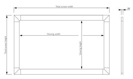
Total frame width = Viewing width + 200mm
